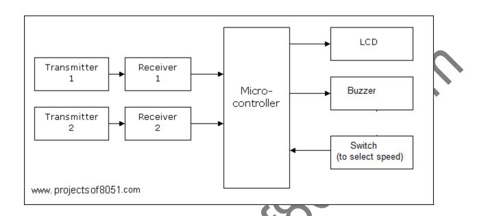
The speed checker for highways implemented here assumes that the maximum permissible speed for highways is either 40Kmph or 60 Kmph as per the traffic rule. Slides switch S1 to select the speed limit i.e. either 40Kmph or 60 Kmph.
